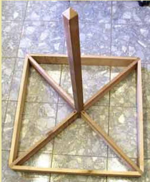
Now attach the supports using one screw in each end. The bottom should look like this.
